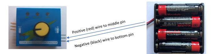
If you have done this correctly you will see the light on the servo motor control unit light up.
