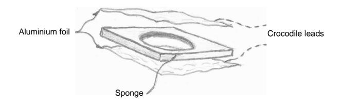
4. You can then put it in your circuit just like a switch and press it to make a bulb or LED light up, a buzzer sound or a motor begin working.
