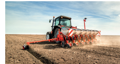
Drill farming equipment (Used to sow seed in the fields)
