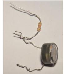
3. Connect the crocodile leads as shown in the diagram. You can use the 0, 1 or 2 ring but this diagram shows the connection between the LDR and the resistor connected to the 0 ring (P0).
